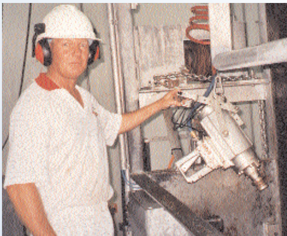
A worker using Jarvis' Model USSS-2 non-penetrating stunner in Valley Beef's Australian processing facility located in Grantham, Queensland.
